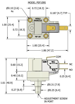
The versatile high-current PSF109S vacuum switch offers
